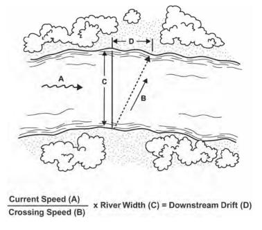
*Note:* The crossing speed for a swimmer across a river may vary but is generally limited to 1 meter per second. All measurements must be in the same unit of measure (e.g., meters, feet).
