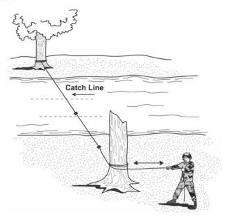
*Note*: The single-rope bridge must be as tight as possible so it will not sag when used.
