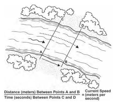
Sight directly across the water from points A and B to locate points C and D.
